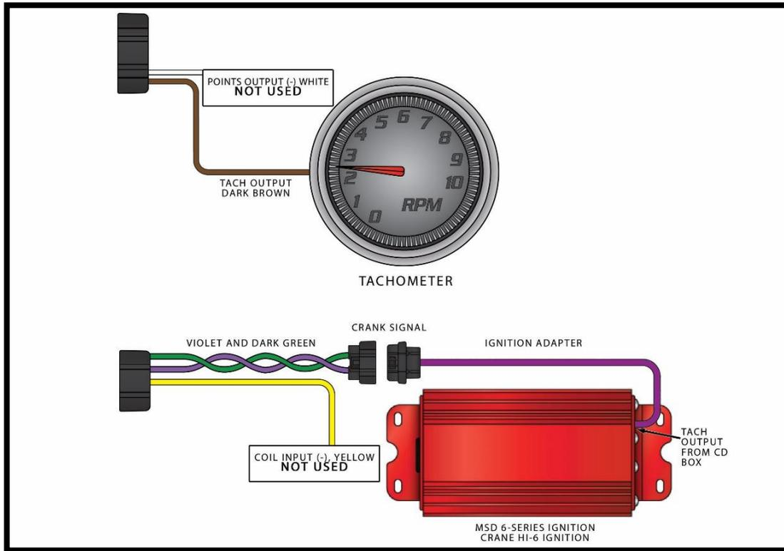
**CAUTION! NEVER connect any of the EFI wires to the coil on any CD type ignition system. The ECU will be permanently damaged!**
